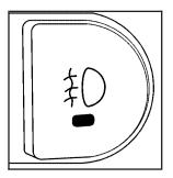
If your vehicle has fog lamps, the fog lamp button is located on the instrument panel, to the left of the steering wheel.
